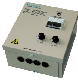
RH-M303A-6/24-C2 [Type housed in case] The base construction is the type installed inside panel. This is placed in a dedicated case to enable installation on the side face of a machine. This type is equipped with a power indicator lamp, voltmeter, magnetic force adjust variable resistor and demagnetizing variable resistor.
