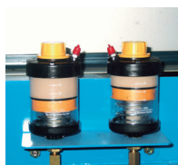
Automatic greasing unit
