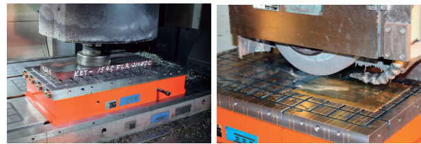
An example of milling by utilizing the permanent electromagnetic feature
